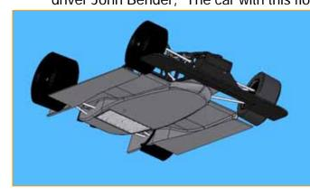
floor works exactly as it was engineered to do. The car has considerably more overall grip, it is less pitch sensitive and has less under steer due to the change in center of pressure, resulting in a well balanced car. This is a whole new level of sportsracer performance."
